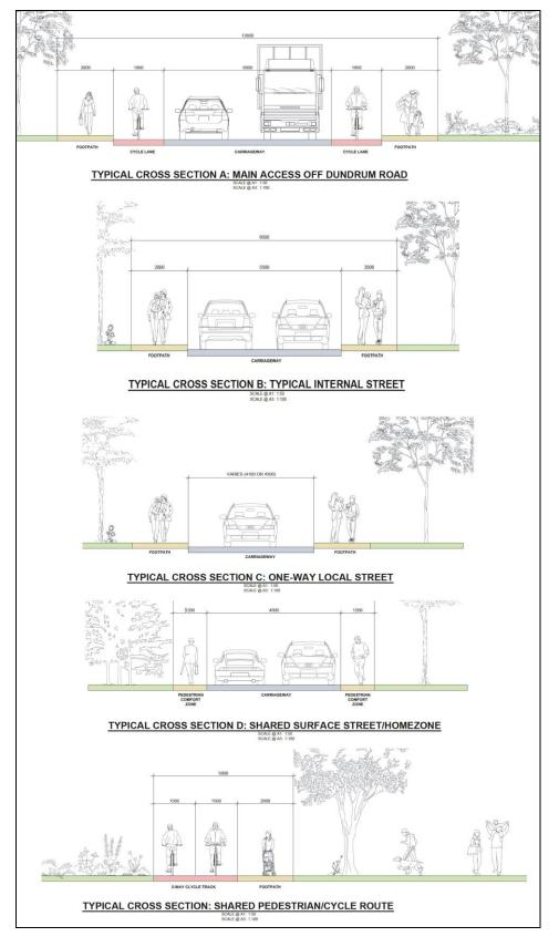
**Figure 3.3: Proposed Cross Sections of Various Streets within SHD Development** (Source: BMCE & Reddy Architecture + Urbanism)
